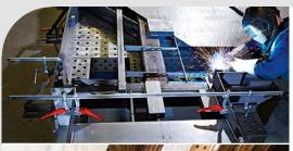
Alongside complete assembled high-performance clamping sets BESSEY also offers versatile accessories that can be combined with one another. Sliding arms that are already fitted can be changed over from clamping to spreading or replaced by different sliding arms or even supplemented with others.
